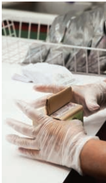
Above, the powdered paint formula is first mixed to establish the correct consistency. Then mineral pigments are added by weight to achieve the correct color. Finally, each bag is packed and sealed by hand. The finished product hits shelves in an earth-friendly brown paper sack.
